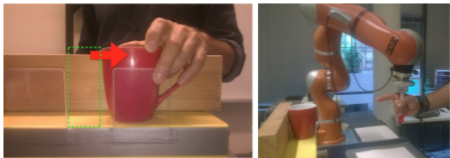
Fig. 1 - left panel: The cup to be rejected is presented to the participant through a narrow window (this picture shows the participant's view). Typically, participants make contact with the point on the cup's rim where the tangent to the rim is parallel to the direction of approach - right panel: The participant contacts and pushes the cup by the extended index finger, while holding a handle mounted on a robot for simultaneous pose and F/T measurement.
