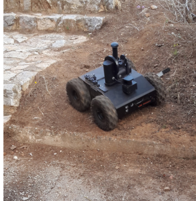
Fig. 1. A DrRobot Jaguar 4x4 robot can be teleoperated to climb a step.
