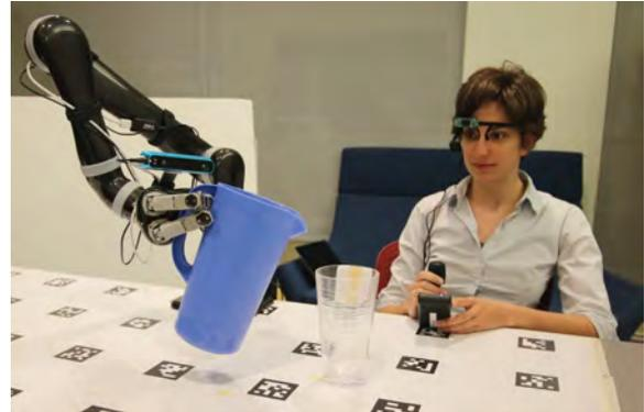
**Figure 1: Eye gaze detected in real time through a head-mounted eye tracker can reveal intentions and guide robot behavior in human-robot collaborations.**
